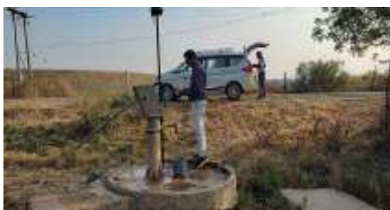
Figure 24: Some photographs of the DGPS survey carried out to determine elevations of the ground water level measurement locations
