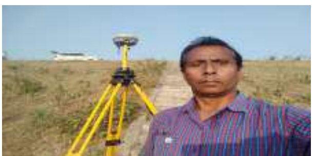
Figure 24: Some photographs of the DGPS survey carried out to determine elevations of the ground water level measurement locations
