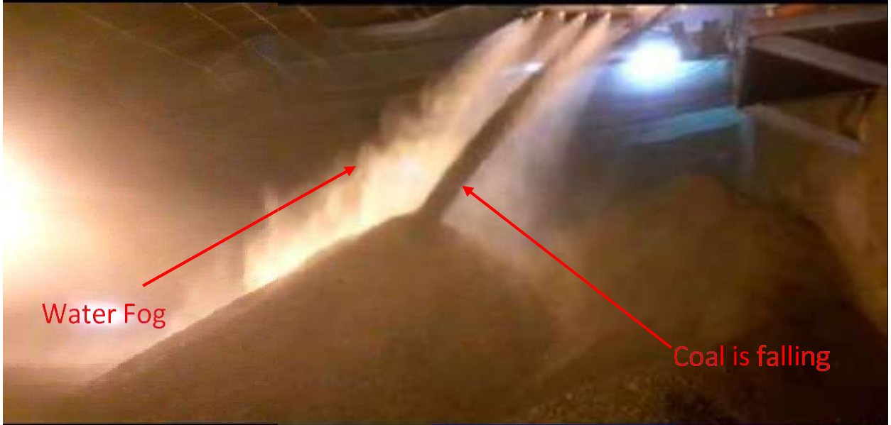
Water Fog over Stacked coal
