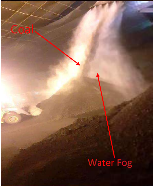
Water Fog over Stacked coal
