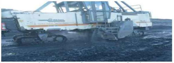
Interlocked Dust Suppression arrangement in Surface Miner
