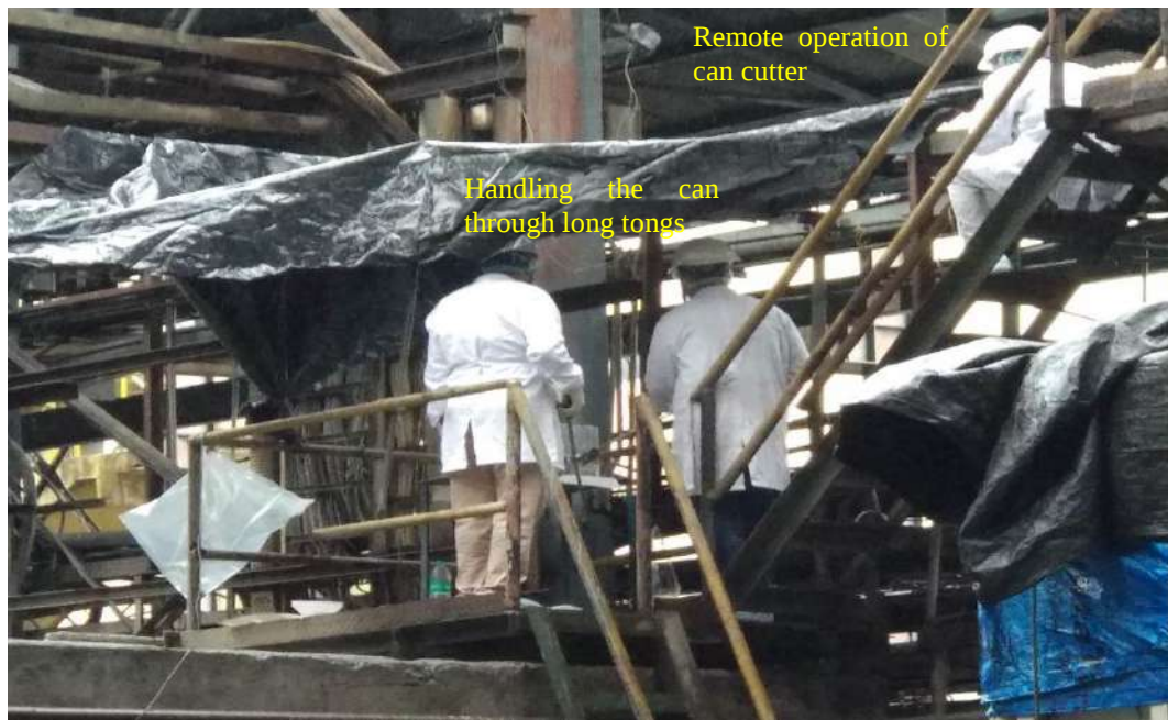
Figure 7: transferring the can in the lead die of can cutter
