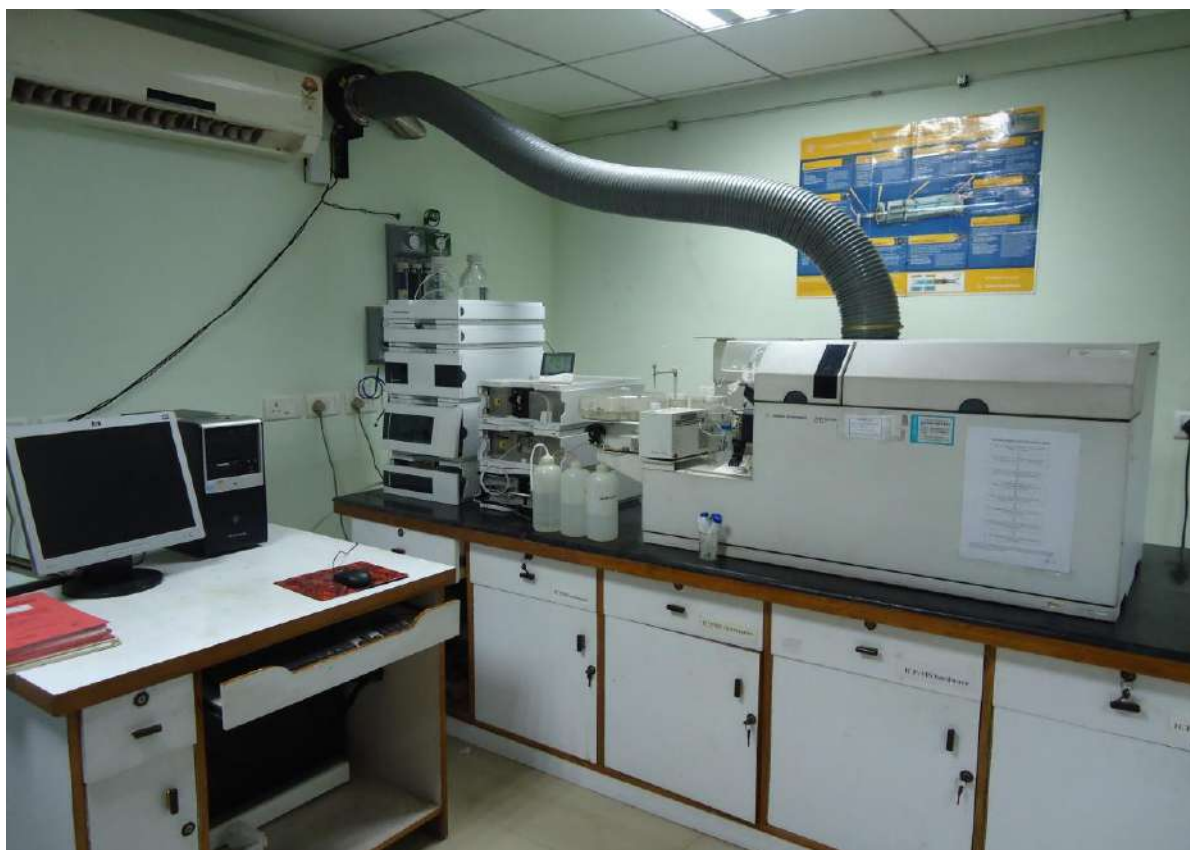
Fig. 3. ICP-MS instrument installed at Central Instrument Facility, used for analysis of various metals.
