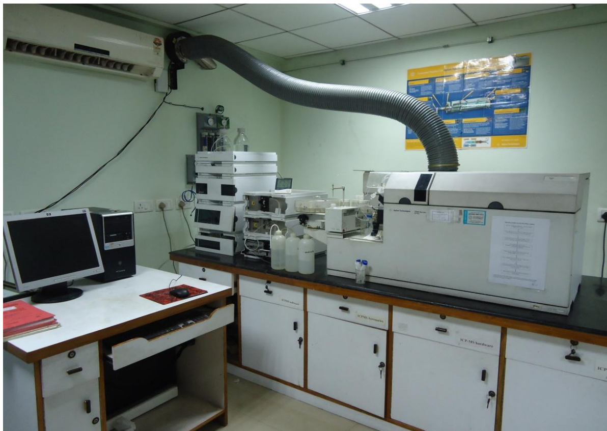
Fig 3. ICP-MS instrument used for metal analysis
