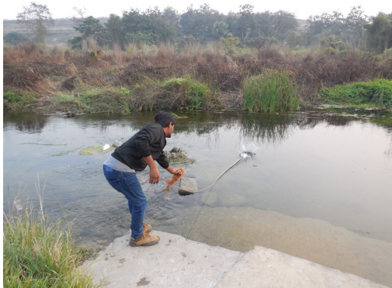
Figure 3.3: Surface water sampling from the Nandra Nala
