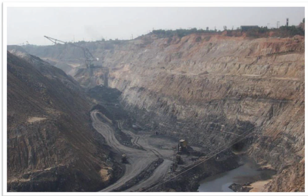
Plate-5.7: Typical Section of Mine Void showing Geological Strata
