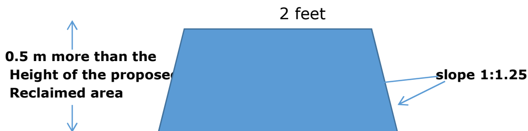
Cross- section of water body protection embankment
